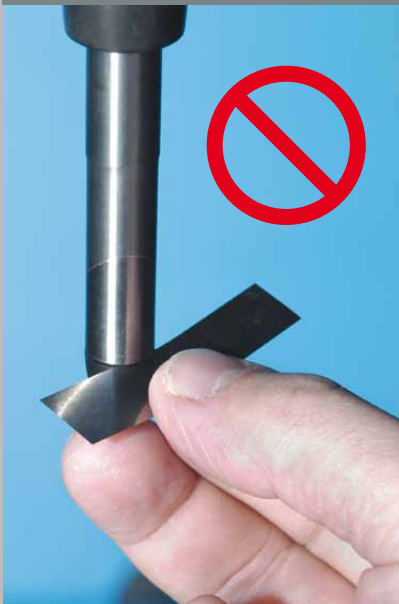
Figure 3a. Shim should NOT enter intersection
