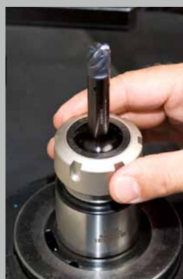
Screw the nut on the holder
