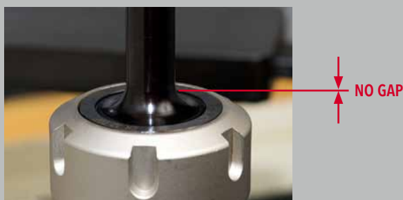
Assemble the nut with the shank by mating the Retention Tabs with the ER Groove
