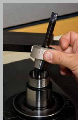
Place the nut/shank assembly into the holder
