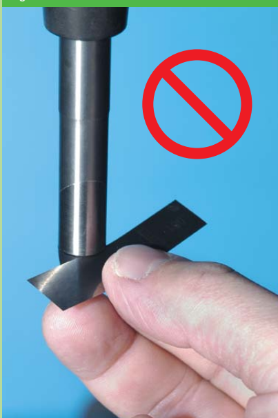
Figure 3a. Shim should NOT enter intersection
