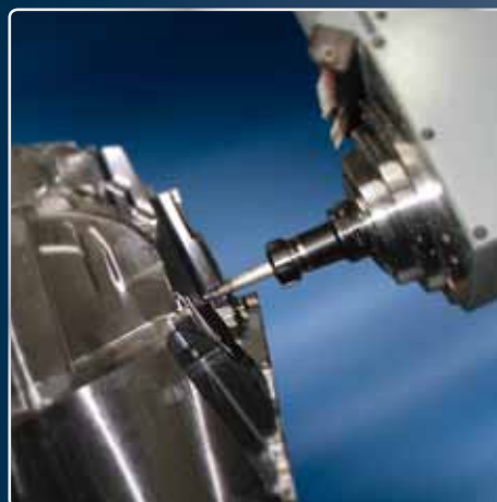
The Ingersoll Chip-Surfer series: Due to easy indexability of the solid carbide heads, several geometries can be applied with only one adaption.
